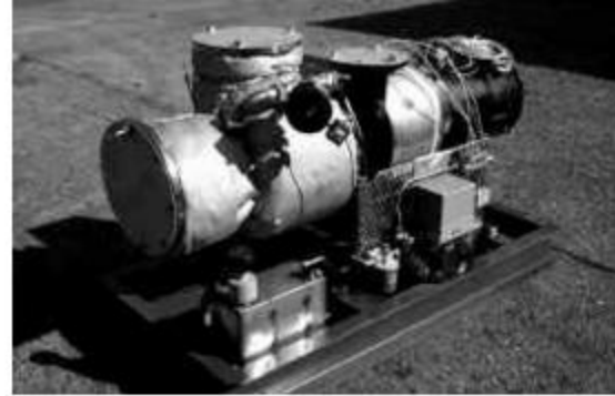
Biomass Turbine Generator
